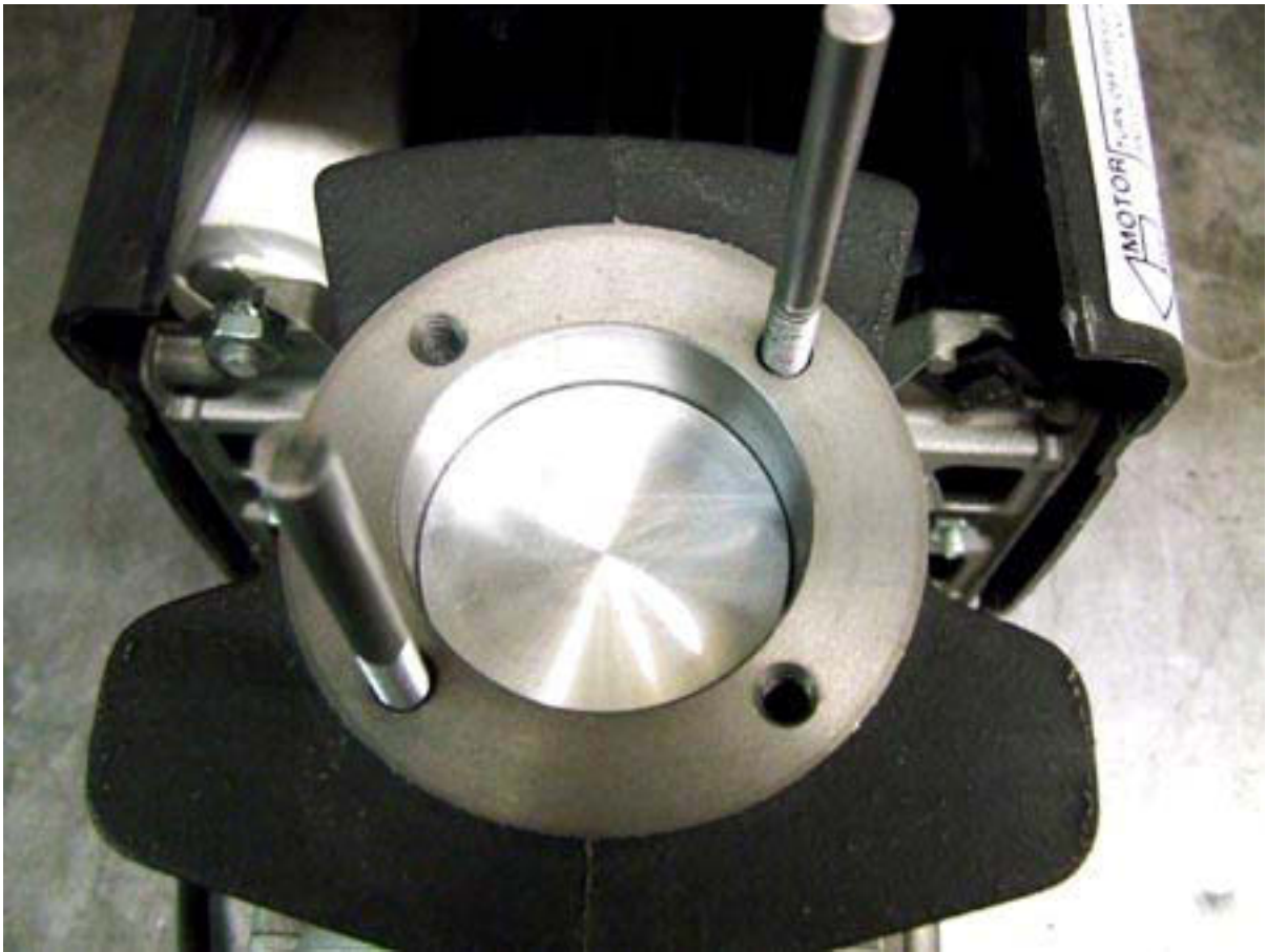
Inserting two studs into the cylinders will assist with alignment
