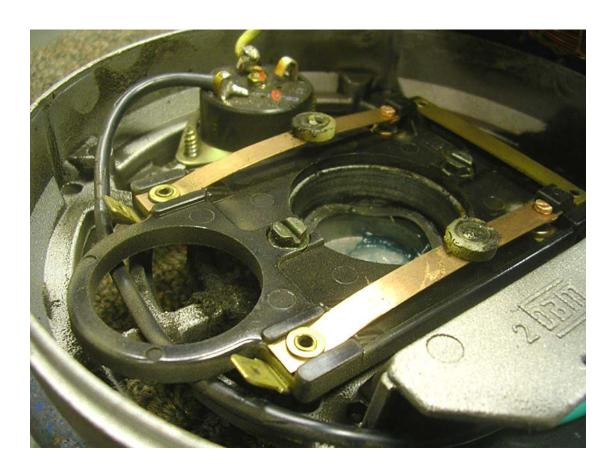
Reassemble the end bell and install the bolts/nuts.
