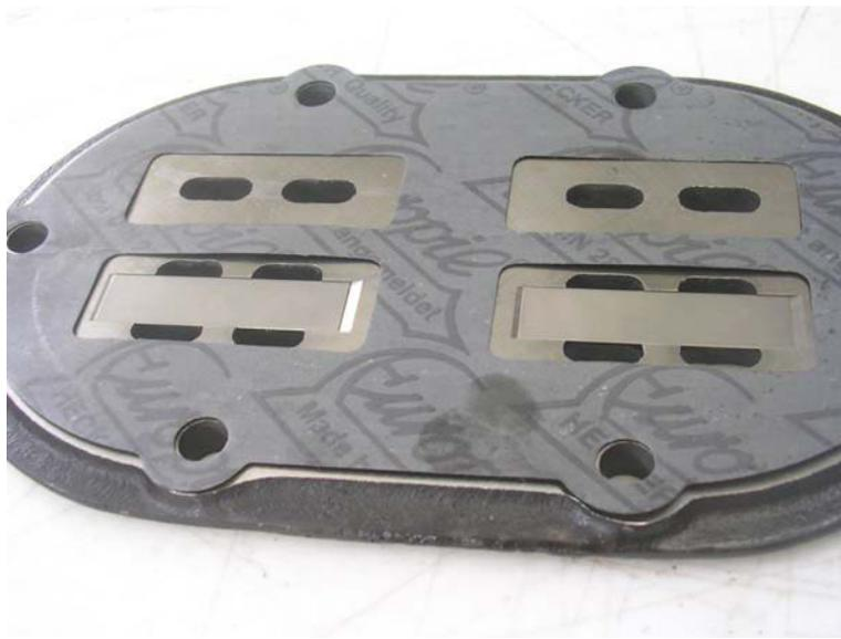
7. Install the valve in the recesses of the second valve plate, using Vaseline to keep them in place, making sure **they do not move**.
