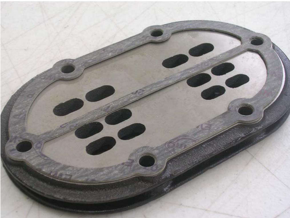
10. Install the pump head and insert head bolts, making sure not to nudge the valve plates or gaskets when doing so.
