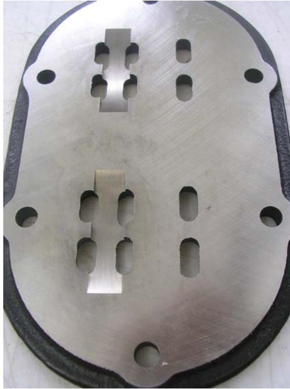
5. Install one valve in each recess, applying Vaseline on the edges of each valve to keep them in place. **NOTE:** Make absolutely sure the valves are installed in the center of each recess and **DO NOT** allow them to move. If they do not stay in place when installing, the pump will not pressurize like it should and could damage the valves.
