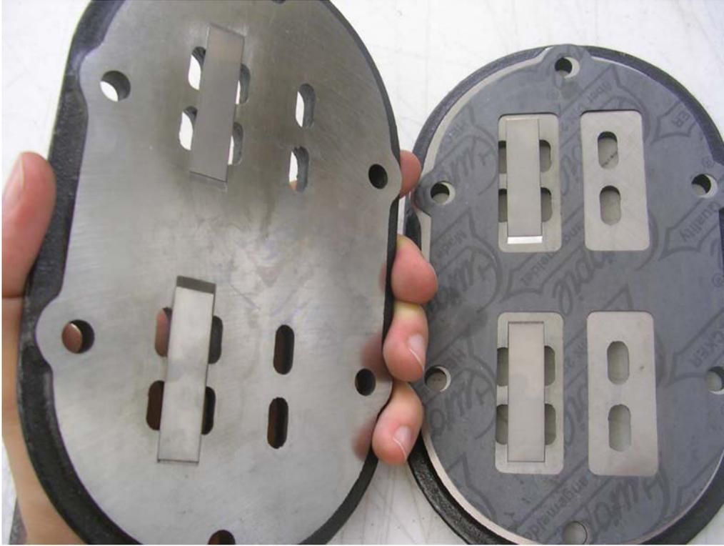
9. Install the Head Gasket (the top gasket in the photo with a rub in the center), again using Vaseline to keep it in place on top of the valve plate.
